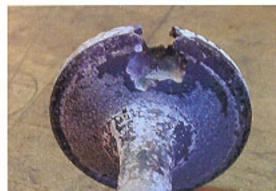
Siloxane damage to a piston head
